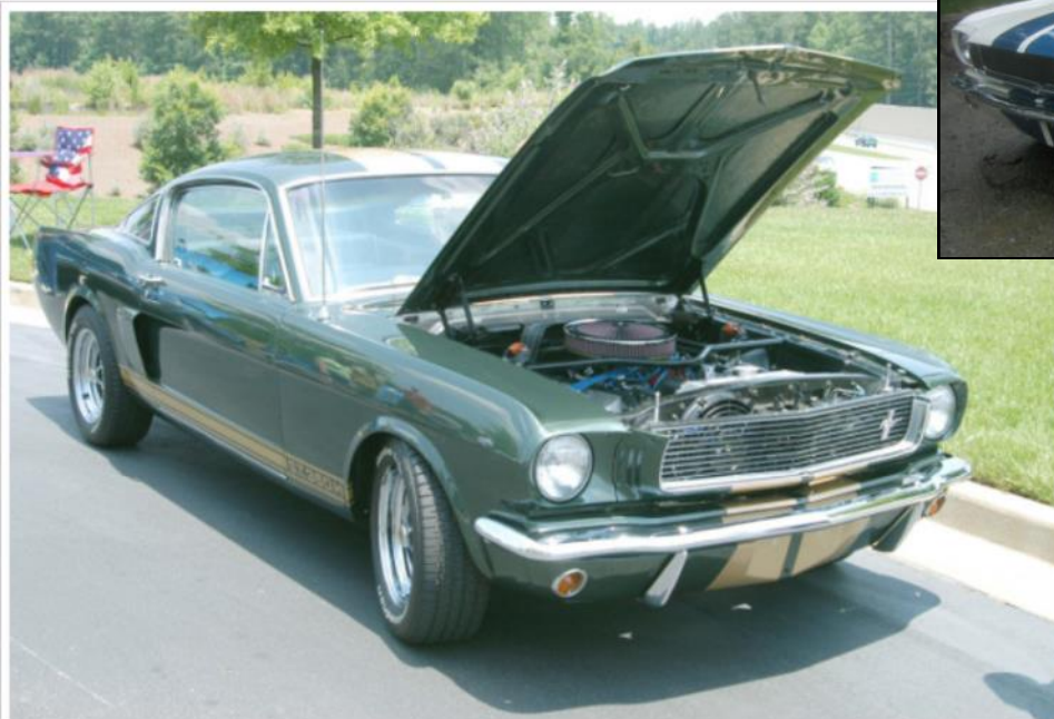
The 1966 Shelby will have a quarter window without the 1965s louvers. Both years have a scoop on the quarter panel.
