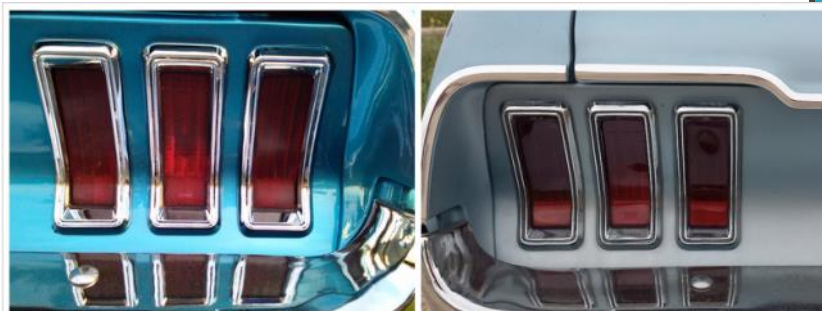
The 1967 tail lamp chrome (left) does not have the black stripe that the 1968 trim has (right).
