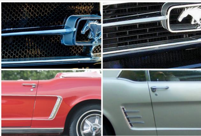
Top: The '64.5 and '65 grille had hexagonal holes, while the '66 grille had horizontal slots, that's a quick way to tell '65 and '66 apart. Bottom: The quarter panel trim on non-GT coupe and convertibles will help distinguish the '66 from the earlier models.
